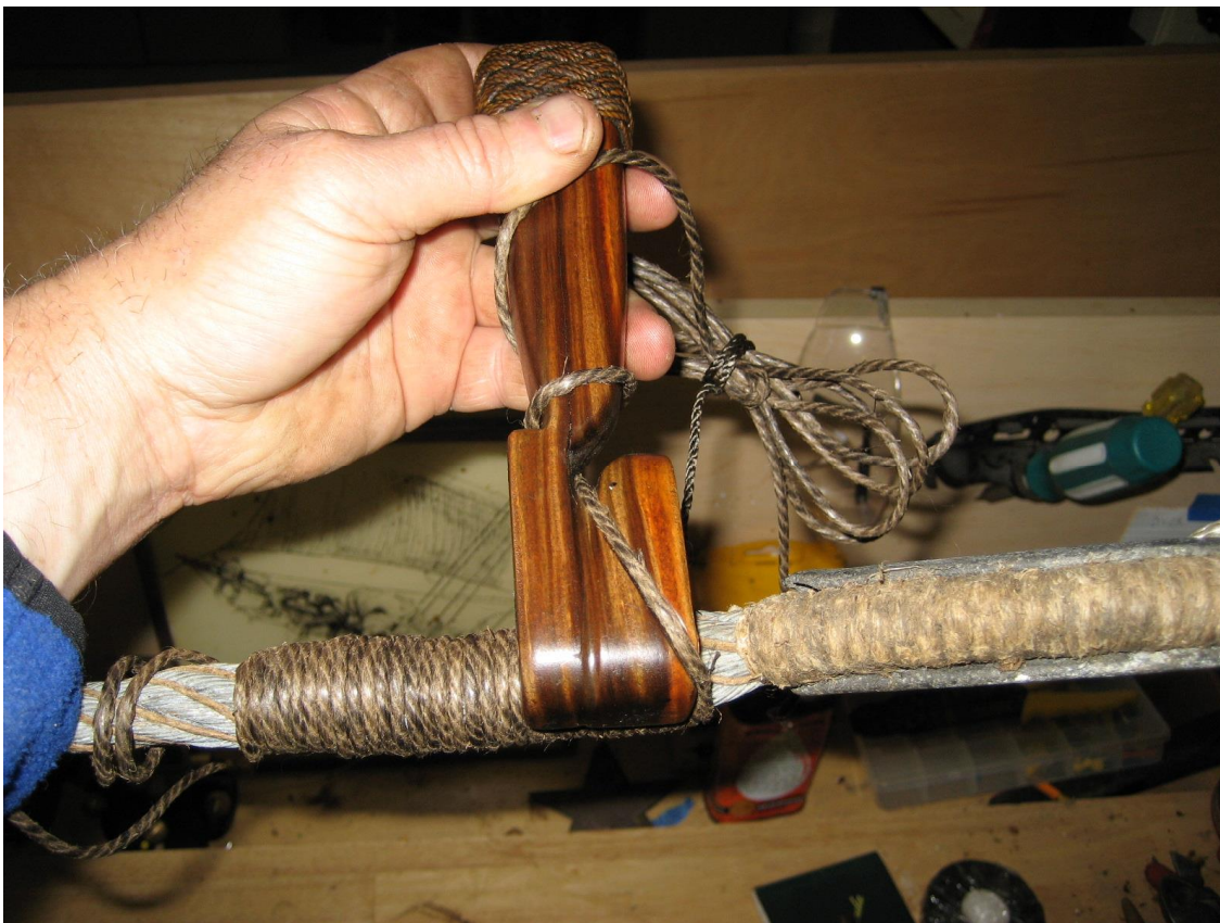
Lignum Vitae serving / seizing board with offset lead in use serving up to a thimble.
