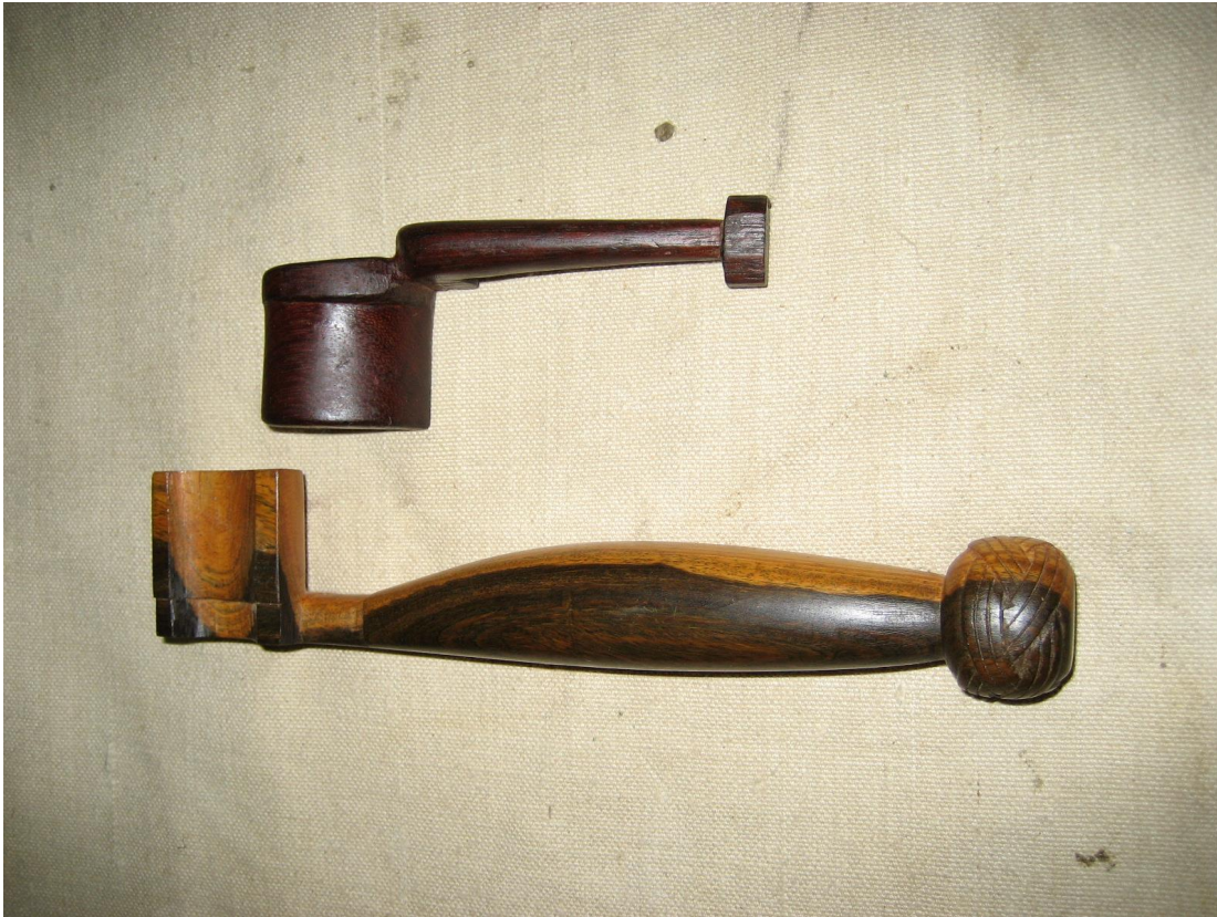
Small Purple Heart palm serving board and larger Lignum Vitae serving board.
