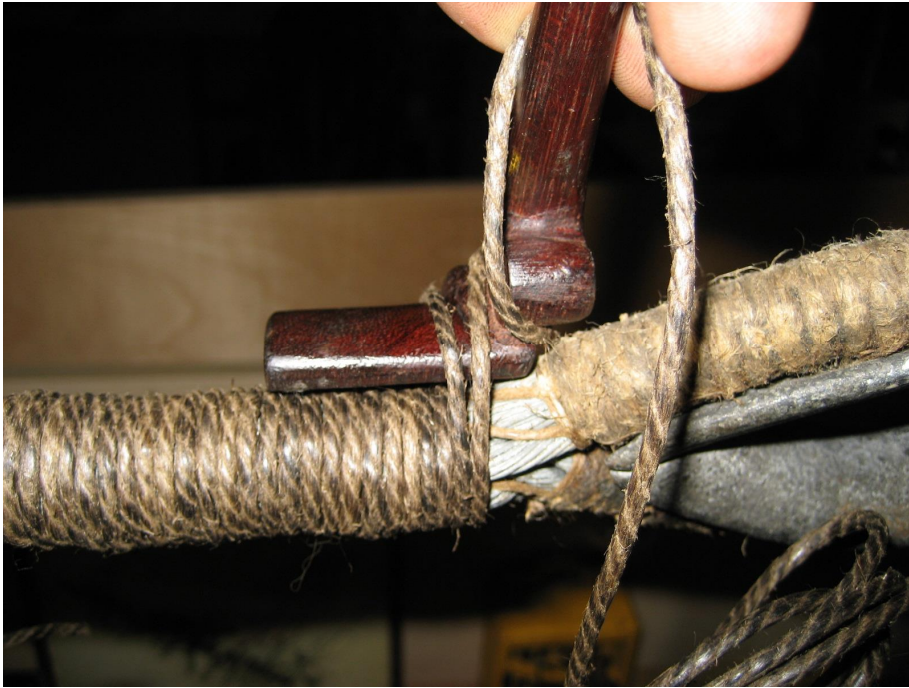
Offset Purple Heart serving board serving up to a thimble.
