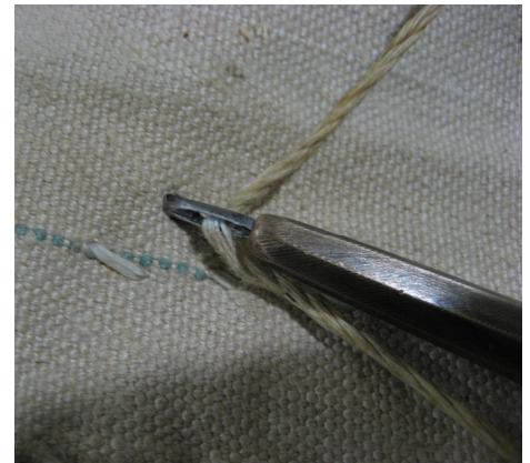
Sailmaker's heaver made out of a bronze bolt with faceted edges to grip the sail twine and a lignum Vitae handle. It works like a capstan and heaves stitches down in heavy canvas. The end has a shallow concave point to seat the head of a heavy needle to push it the last inch or so through the canvas. A very handy tool.
