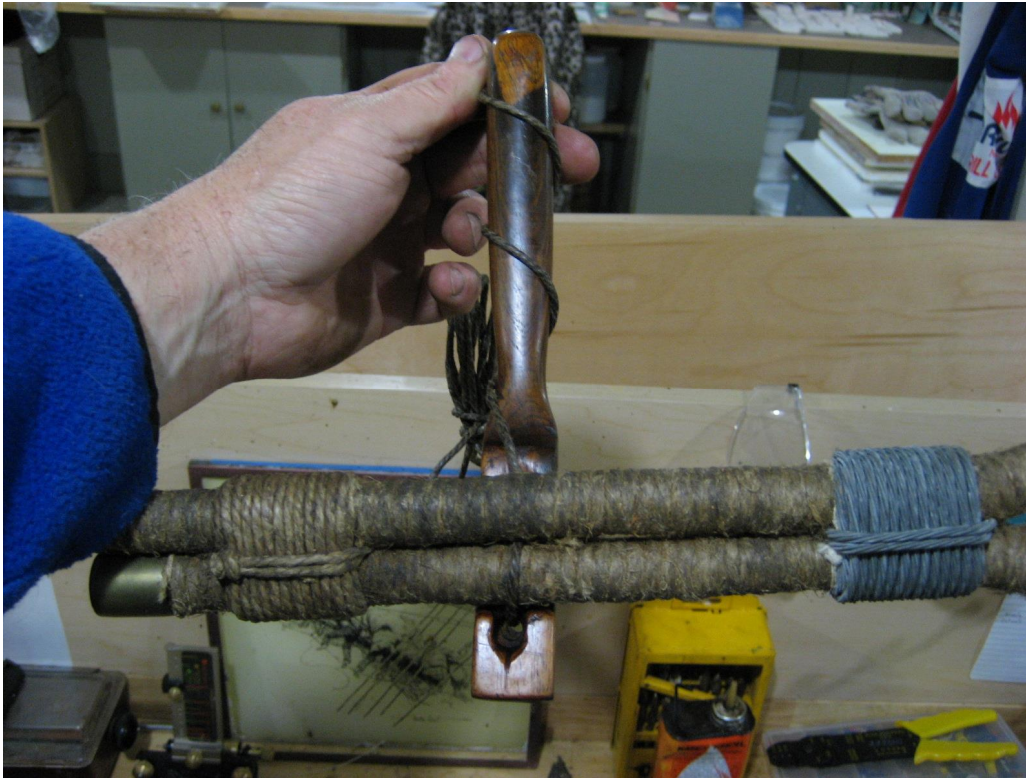
Lignum Vitae seizing stick clapping on a fiber seizing.
