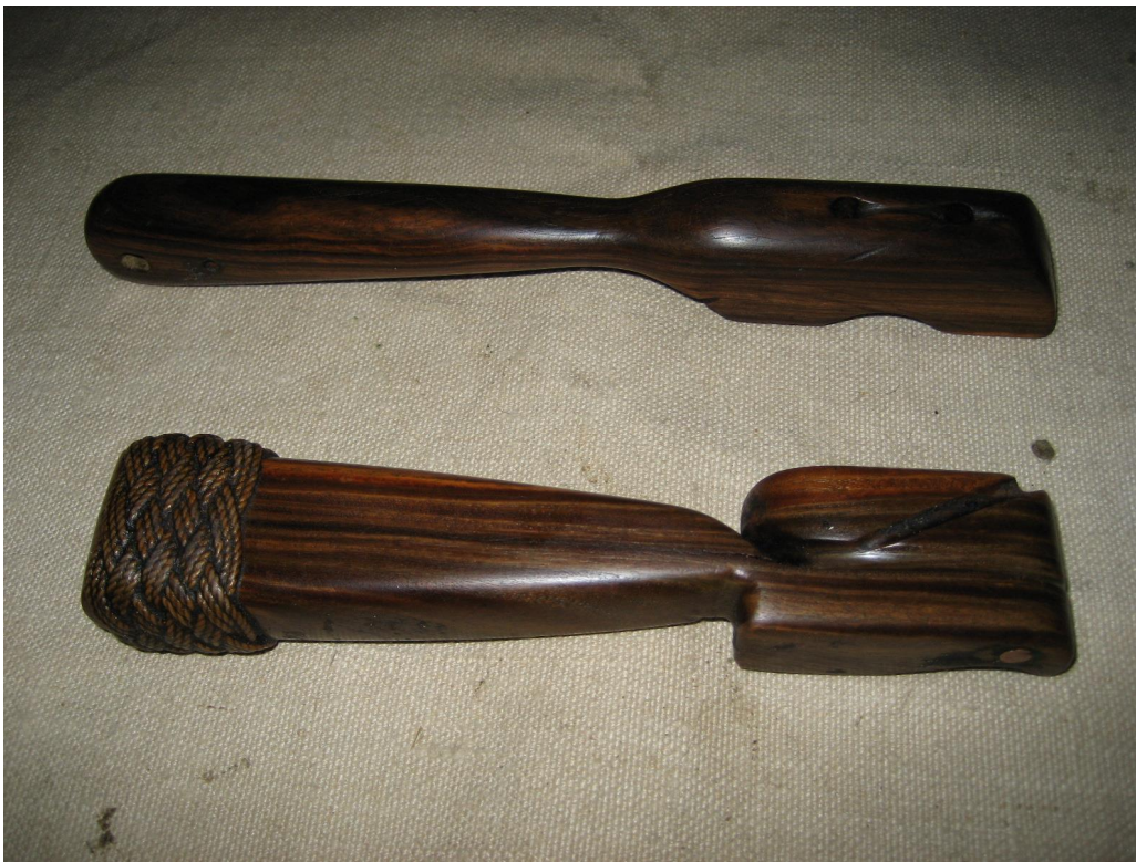
Lignum Vitae serving / seizing boards ñ lower one has an offset lead to serve up to an eye.
