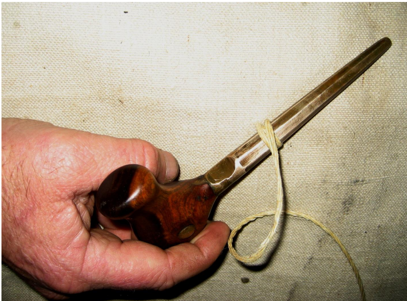
Sailmaker's heaver made out of a bronze bolt with faceted edges to grip the sail twine and a lignum Vitae handle. It works like a capstan and heaves stitches down in heavy canvas. The end has a shallow concave point to seat the head of a heavy needle to push it the last inch or so through the canvas. A very handy tool.
